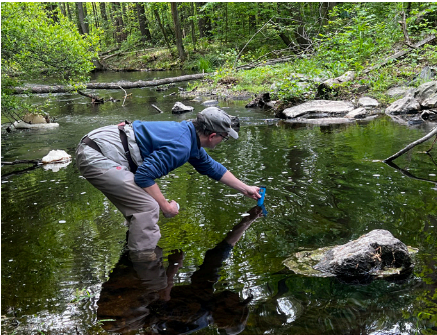
A volunteer uses a hand-held meter to test temperature and conductivity in Catecunemaug Brook just downstream from the Lake Shirley Dam in Shirley, MA. Photo by Gaynor Bigelbach
